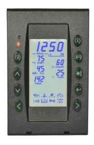
Fully programmable digital control panel suitable for low-power and midpower engines.
