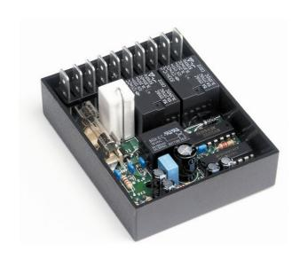
**CT61** is a microcontroller-based control unit for one wiper. It manages both single speed and double speed motors. All functions are performed by a DPDT (double pole, double throw) momentary switch (not provided) with neutral position (On - Off - On).
