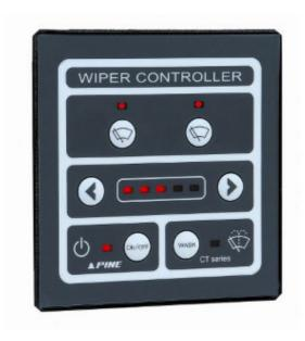
**CT2N2** is a microcontroller-based wiper control system for 2 wiper motors.
